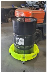
"We benefit from the new CRWP provided euipment in many ways. The pull tray allows us to easily move a full drum of hydraulic all around the shop while containing any unexpected spillage that may occur during equipment filling. The outdoor storage container allows us to keep our oil storage containers protected from the elements, containing any accidental spillage and quite frankly makes the storage of drums look more professional.
