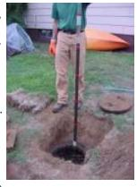
need for septic tank pumping. This will be determined by measuring the depth of septic sludge and scum in the tank.
