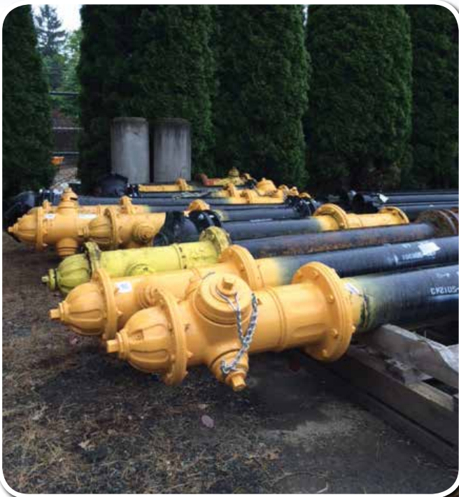
Water system inventory of fire hydrants and ductile iron pipe.
