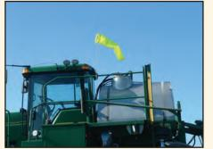
Windsocks are calibrated to indicate wind speed from 2 to 12 miles per hour
